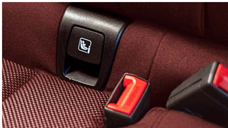
ISOFIX Child Restraint System is located at the rear that allows appropriate securing of child safety seat.
