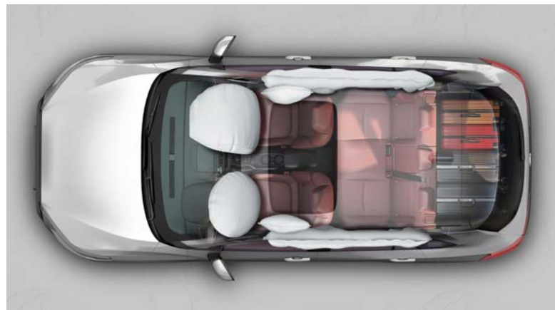
7 SRS Air Bags provide protection to the driver as well as the passengers in case of emergency.
